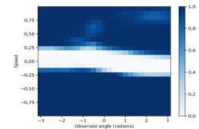
The agent takes accurate samples when the observed position of the pendulum is close to the upright position and hence the speed is low:
